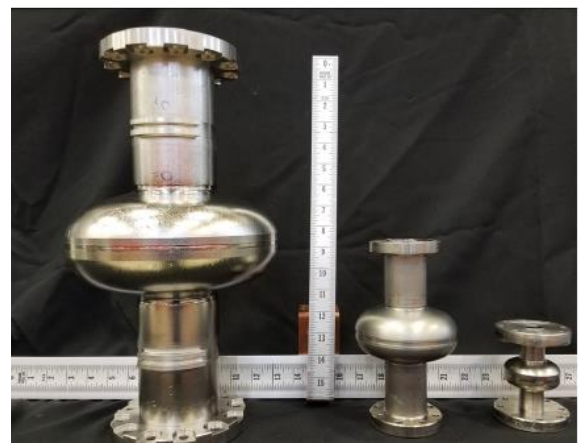
Single - cell cavities measured for Q at low temperatures. From left to right, the frequencies are 1.3, 2.6 and 5 GHz.
